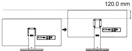
The height can be adjusted up to **130.0 mm**.
