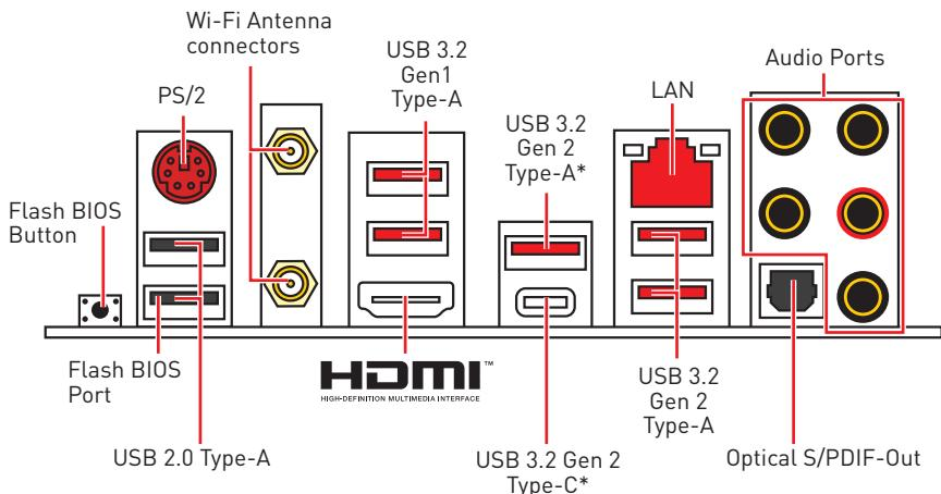
\*USB 3.2 Gen2 (3rd Gen AMD Ryzen™) or USB 3.2 Gen1 (2nd Gen AMD Ryzen™/Ryzen™ with Radeon™ Vega Graphics and 2nd Gen AMD Ryzen™ with Radeon™ Graphics)
