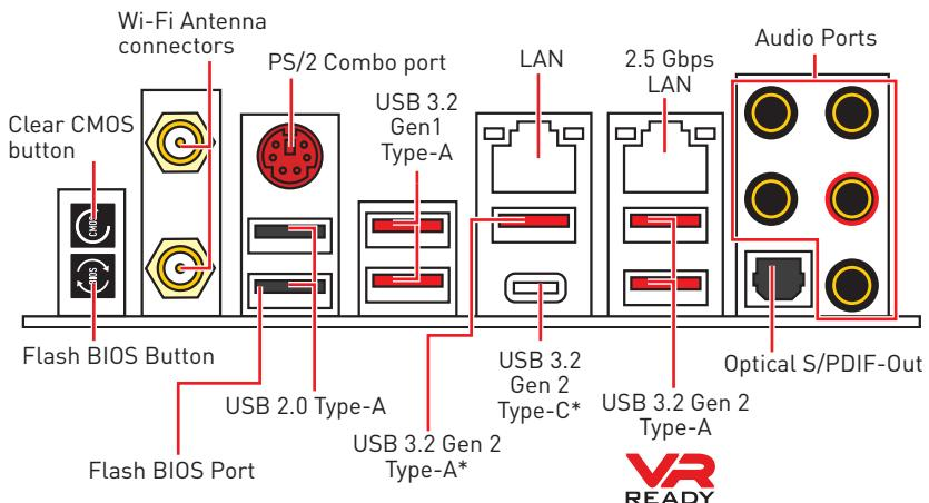
\*USB 3.2 Gen2 (3rd Gen AMD Ryzen™) or USB 3.2 Gen1 (2nd Gen AMD Ryzen™/Ryzen™ with Radeon™ Vega Graphics and 2nd Gen AMD Ryzen™ with Radeon™ Graphics)
