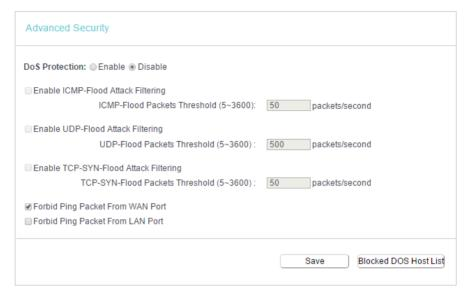
DoS Protection - Denial of Service protection. Select Enable or Disable to enable or disable the DoS protection function. Only when it is enabled, will the flood filters be enabled.
