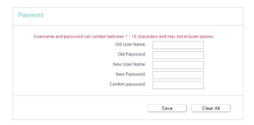
It is strongly recommended that you change the default username and password of the router, for all users that try to access the router's web-based utility or Quick Setup will be prompted for the router's username and password.
