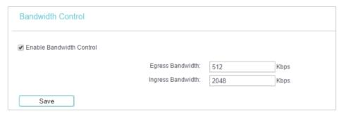
The values you configure for the Egress Bandwidth and Ingress Bandwidth should be less than 100,000Kbps. For optimal control of the bandwidth, please select the right Line Type and consult your ISP for the total egress and ingress bandwidth.
